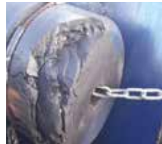
Damaged part rebuilt
